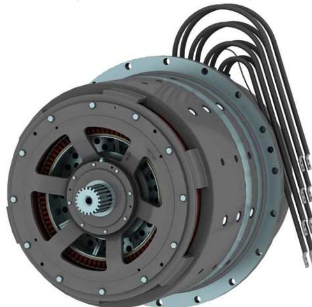
Figure 2 – Design of EDP-800 traction motor
