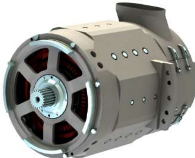
Figure 2 – Design of EDP-600 traction motor (drive-side view)
